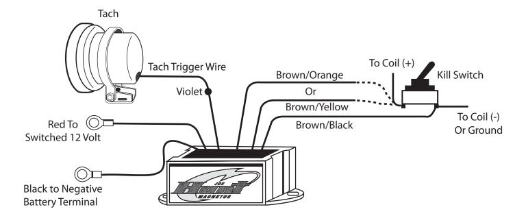
**Tip:** For Super Mag applications it is recommended that ground straps be connected from both cylinder heads to the magneto clamp.
