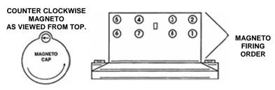
**NOTE:** NUMBERS ON MAGNETO CAP INDICATE FIRING ORDER OF MAGNETO ONLY
